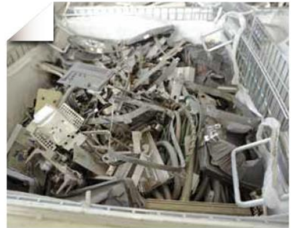
Industrial VLLW (such as scrap metal and plastics) before conditioning
